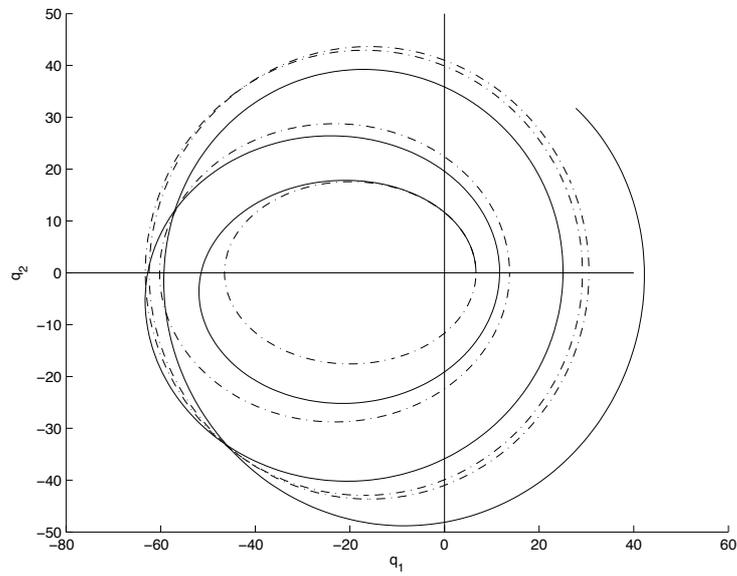
**Fig. 1.** Energy minimizing transfer towards the geostationary orbit, final time  $t_f = 19.290$  hours. The trajectory is the solid line that osculates the dashed intermediary orbits of the averaged system.
